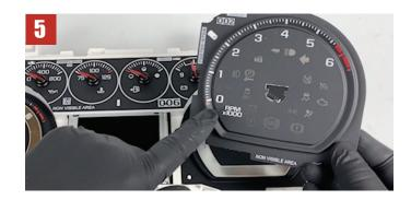
(Image 6) Be careful to leave room between the needle hub and the gauge face. Check to make sure the needle is in the same relative position as previously marked.
