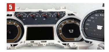
(Image 6) Be careful to leave room between the needle hub and the gauge face. Check to make sure the needle is in the same relative position as previously marked.
