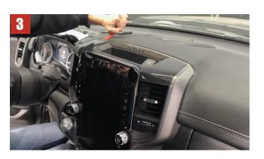
Be aware, the electrical cable supplying the axillary/lighter receptacle is connected. You may remove this if you choose. The unit will sit in the center console without disconnecting this cable.
