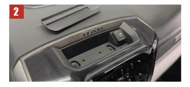
(Image 3) Next, remove the entire unit. To do this, gently insert your trim removal tool at the top of the unit in the seam between the unit and dash. Pry gently to start to remove it from its clips. Gradually work your way around the top of the unit. Once the top clips are free, you should be able to free the rest of the unit by pulling back on it.
