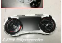
7. Remove OEM gauge face from the cluster and replace it with your new US Speedo, custom gauge face
