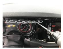
2. Remove screws that hold instrument cluster into place
