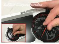
8. Press needles back onto stepper motor and rotate counter clockwise again, making sure you stop the needle at its original location marked on OEM part
