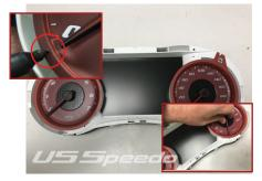
5. Mark the factory needle set with marker on OEM gauge face as shown in the picture
