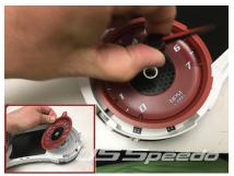
6. Once needles are marked, rotate speedo and tach counter clock wise and pull straight up on needle to remove it from stepper motor
